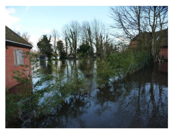
High groundwater levels are likely to have contributed to the flooding of houses in Churchmere Road in 2014, in combination with drainage of surface water from the landfill site into the nearby lake (see photo above).
